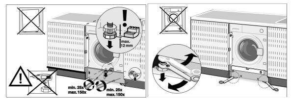
The water intake and drain hoses can be fitted pointing to the left or right for effective installation.
